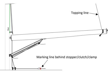
A system that is set to the correct angle and operated correctly will result in a moderate amount of pull back and keep the mainsail luff nicely taut.
