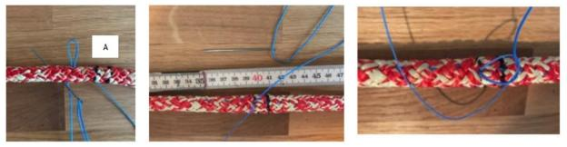
Secure the middle of the splice with some stitches. I am using regular 1mm waxed polyester whipping line. I like to finish it by making a simple" half knot", burying the ends and then cutting them. <u>We recommend turning the rope 90 degrees and repeat the operation.</u>
