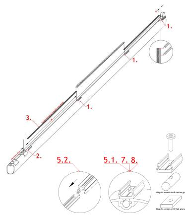
3. If the Sunbrella does not fit or if there is not any sail groove on the mast, a support rail is necessary to install on the mast. Place the subrail to the support-rail in extension of the POMramp and mark the end and the position of the holes for drilling.
