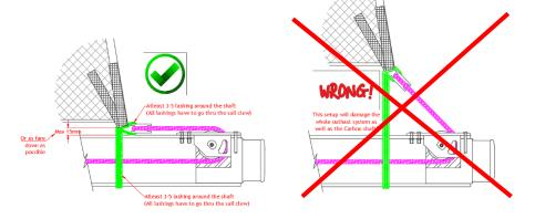
Before using the outhaul system! We recommend to tighten foot so it runs paralle with the shaft. Place a MARK on the mast, out from the position of the low friction ring. This will help indicate when to STOP, and minimize the risk of damaging the Outhaul system or the sail.
