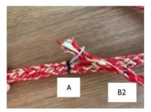
Pull the end of the cover until both points A are aligned. Repeat for other side.
