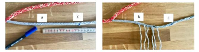
Thin out the core at point B. (The core will eventually be cut at C and thinned out all the way there. At this point I recommend taking out only 5 or 6 strands to facilitate Step 4, while keeping the structure of the braid.)
