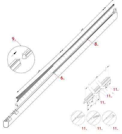
11. When the mast-rail is properly placed, drill the holes and thread in the sub-rail. Make them through the pre-drilled holes in the mast-rail. The holes are placed in both ends and in the middle of the mast-rail, on each part of the mast-rail. Use the supplied drill and the thread-tapping tool to make the holes and the threads. Use the supplied screws to attach the mast-rail to the sub-rail.
