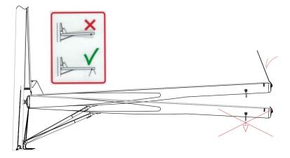
Note! With numerous uncontrolled "jibs" will there be the possibility of damaging the boomtoggle joint. It's therefore always the user's responsibility to be aware of his surroundings and to secure the boom correct, so that the boom can't sway uncontrollable.
