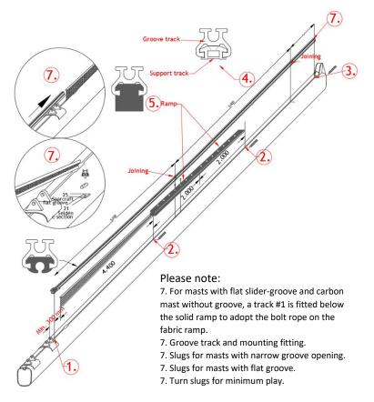
If any adjustments are needed to be made, we recommend to this at upper joining.
