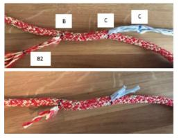
Cut the end of the cover at B2 and cut the core at C. Thin out evenly by cutting the individual strands in different places.
