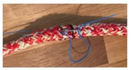
Step 6: Cut & taper the core and cover
