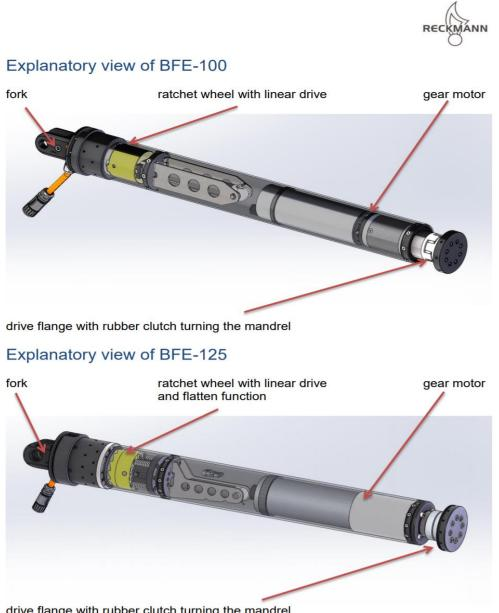
drive flange with rubber clutch turning the mandrel
