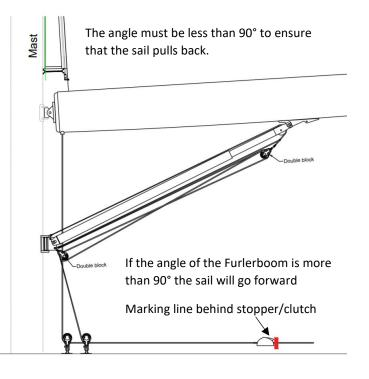
with a thicker tail by the clutch, and a mark needs to be set to correspond with the boom in the correct position for furling. We recommend that a mark is made on the line, such that it is easy to see and to reproduce every time you wish to furl.
